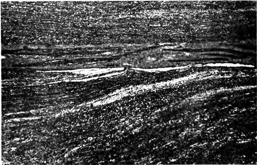
Fig. 12 (Investigation 135-16)—Photomicrograph showing a different area of the same shelly crack shown in Fig. 10. It can be noted that a gray (iron oxide) and white (unidentifiable) foreign material are present in this work-hardened metal. Magnification, 500X. Etchant, 3 percent nital.
